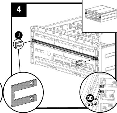
Note: Countersink on bracket must face inside of cabinet on both sides. See inset for proper part orientation.
