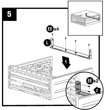
Attach Hanging Bracket (L) to back panel using four screws (EE). Attach (L) to side panels using four screws (EE). Mount cabinet to the wall as shown in the following steps, before assembling lid.
