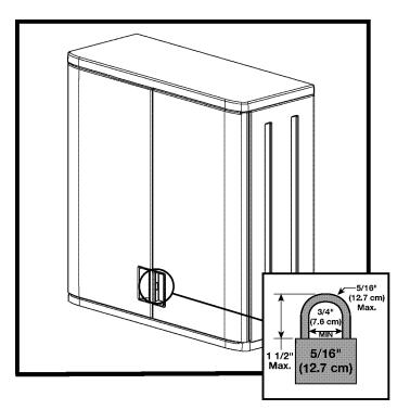
With doors closed, attach a 5/16" lock (not provided).
