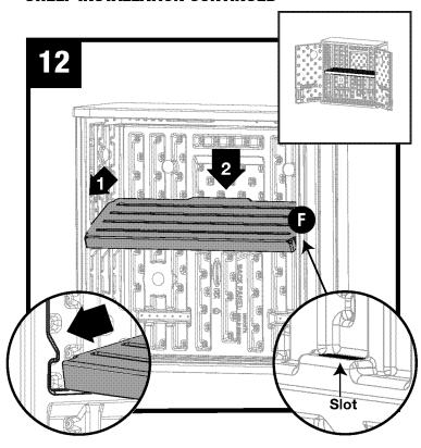
Tab on shelf must engage with slot on inside panel. Push side panels inward to engage.
