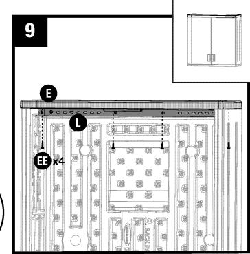
Attach top panel (E) to top of bracket (L) using four screws (EE).
