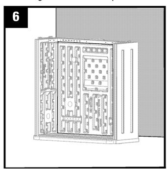
Place cabinet in desired location. Determine desired height and mark with a horizontal line. Line up bottom of cabinet with this horizontal line. Note: Top will be attached after wall mounting.
