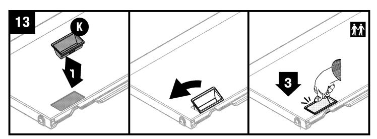
Place door on a flat hard surface. Lower (K) into left door. Insert on an angle. Hole for lock must be facing inside of cabinet. Push down hard on center of handle to snap in place. Repeat with right door.
