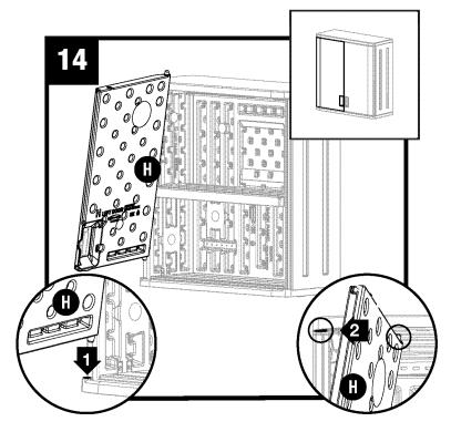
With left door (H) in the open position, place door into hinge receptacle on bottom left of cabinet. Insert hinge pin under top panel and slide to the left into hinge receptacle. Repeat with right door (G).
