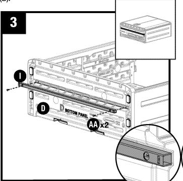
Attach support tube (I) to bottom panel (D) using two screws (AA). Large hole of support tube must face out.
