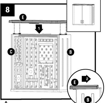
Make sure all tabs are engaged before locking panels together.
