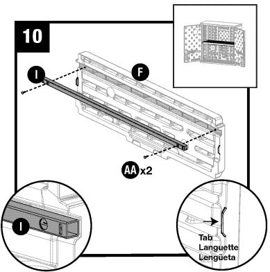
Attach support tube (I) to shelf (F) using two screws (AA). Large hole of support tube must face out.
