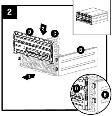
Align and engage slots on bottom panel (D) with tabs on side panels (C) and (B). Push down until you hear a "snap" to lock in place.
